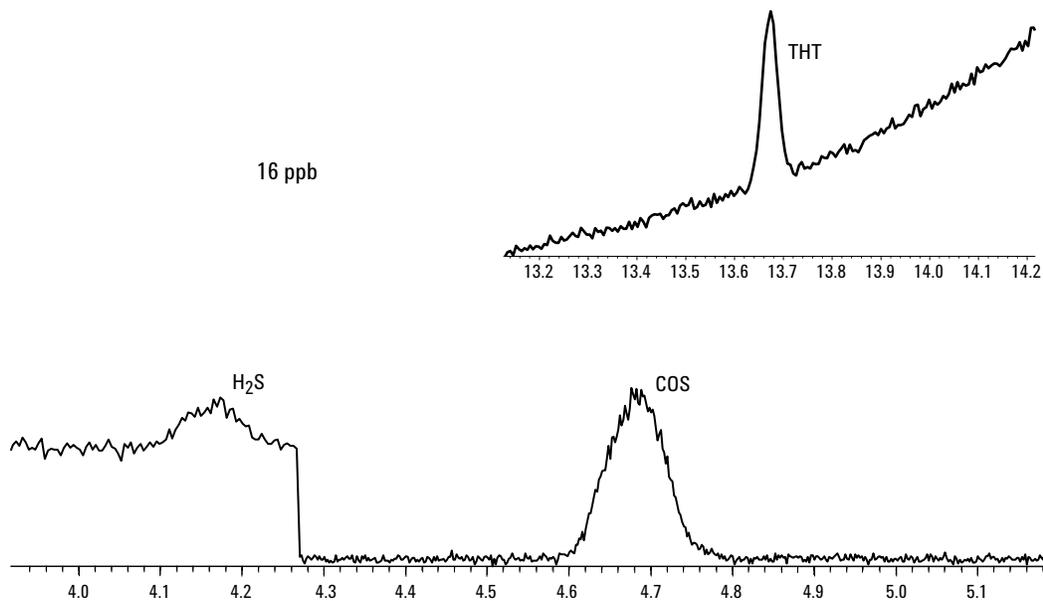
**Figure 7. H<sub>2</sub>S, COS and tetrahydrothiophene (insert) at 16 ppb each. SIM was used.**
