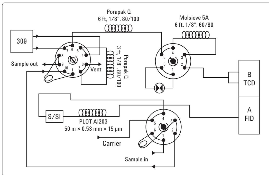
Figure 1. Valve diagram for dual-channel natural gas analysis.
