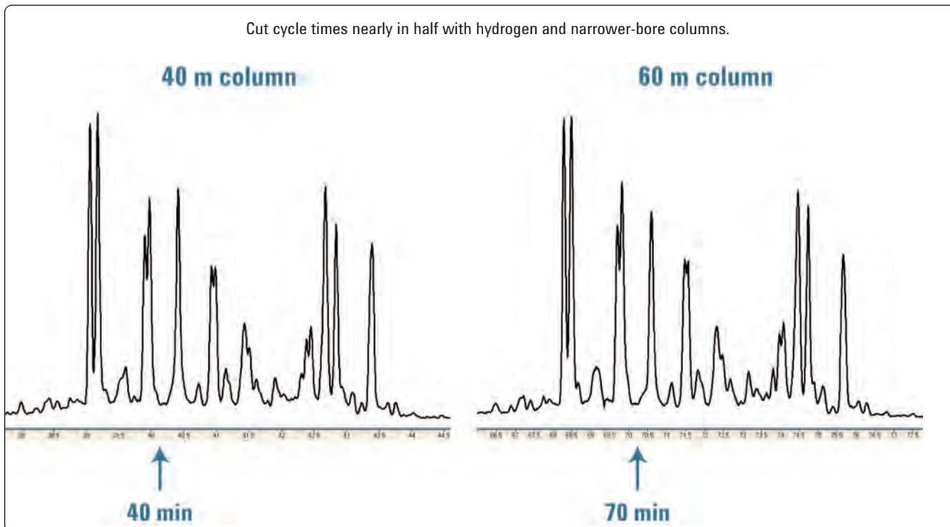
Figure 3. C28 steranes were analyzed using  $m/z$  transition 386→217 on either a 60 meter, 0.25  $\mu\text{m}$  column and helium carrier gas, or a 40 meter, 0.18  $\mu\text{m}$  column with hydrogen carrier gas. Employing hydrogen and the smaller bore column reduces analytical time significantly without loss in compound resolution.
