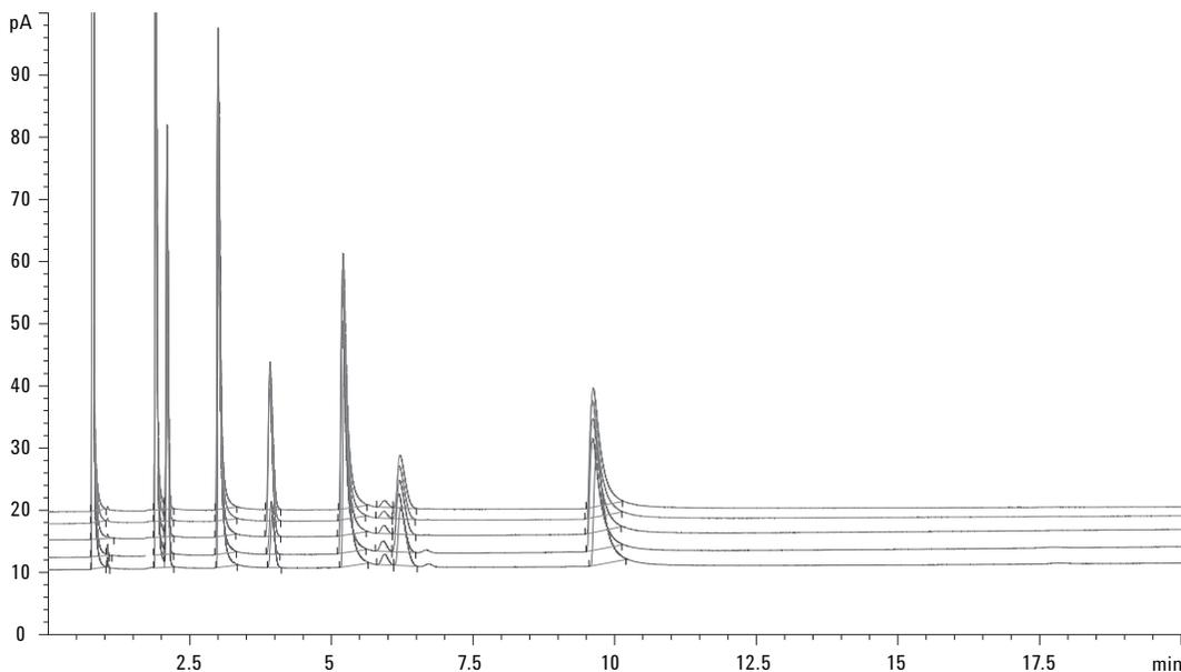
**Figure 5. Fifth run overlaid using GS-OxyPLOT (after conditioning column).****Table 7. Peak Area Reproducibility and Retention Time Reproducibility on GS-OxyPLOT (after conditioning column)**
