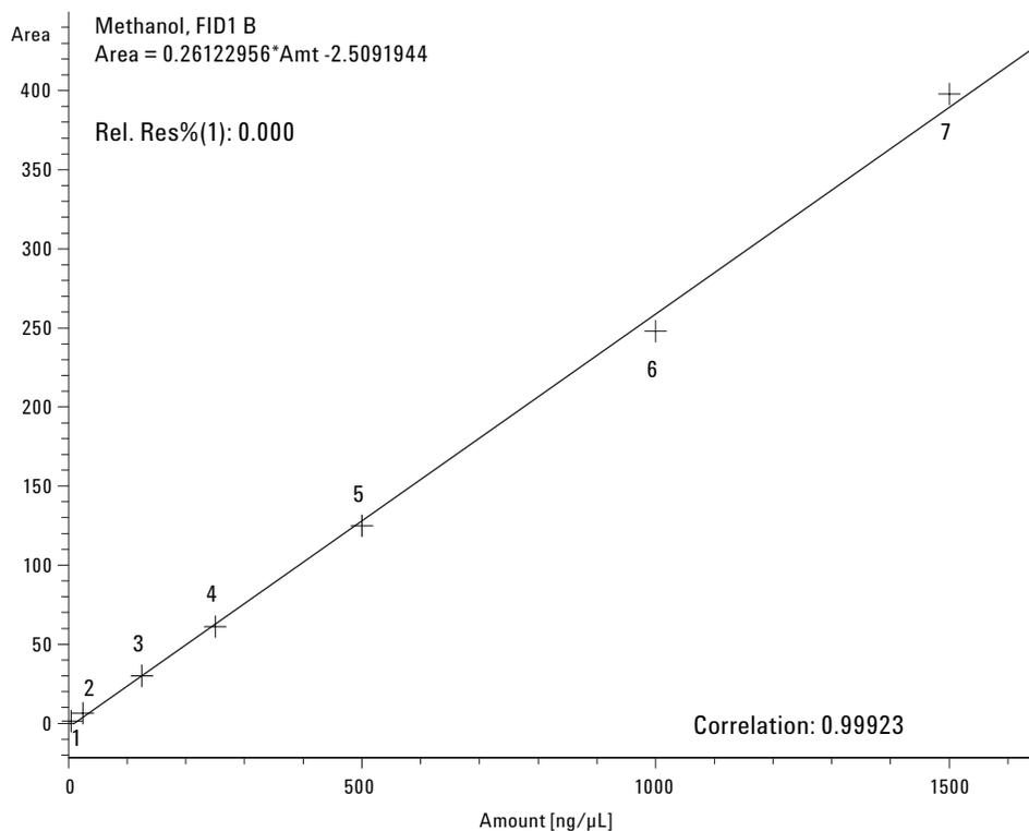
**Figure 6. The calibration curve of methanol in toluene.**
