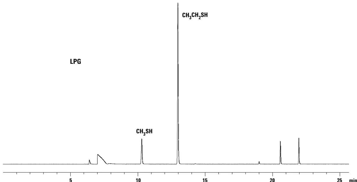
Figure 11. FPD analysis of LPG showing ethyl mercaptan at 2.5 ppm.
