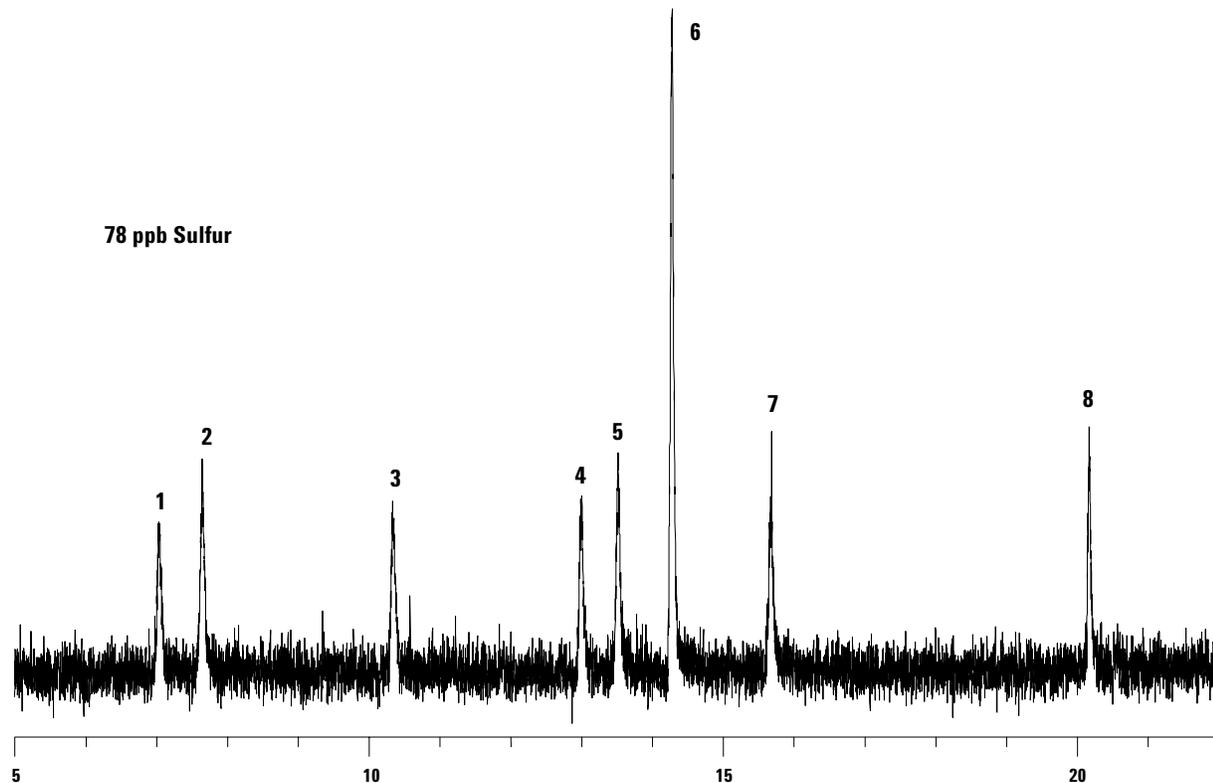
**Figure 4. Eight volatile sulfur compounds at 78 ppbv per component. Detector - Flame Photometric. See Table 3 for peak id's.**
