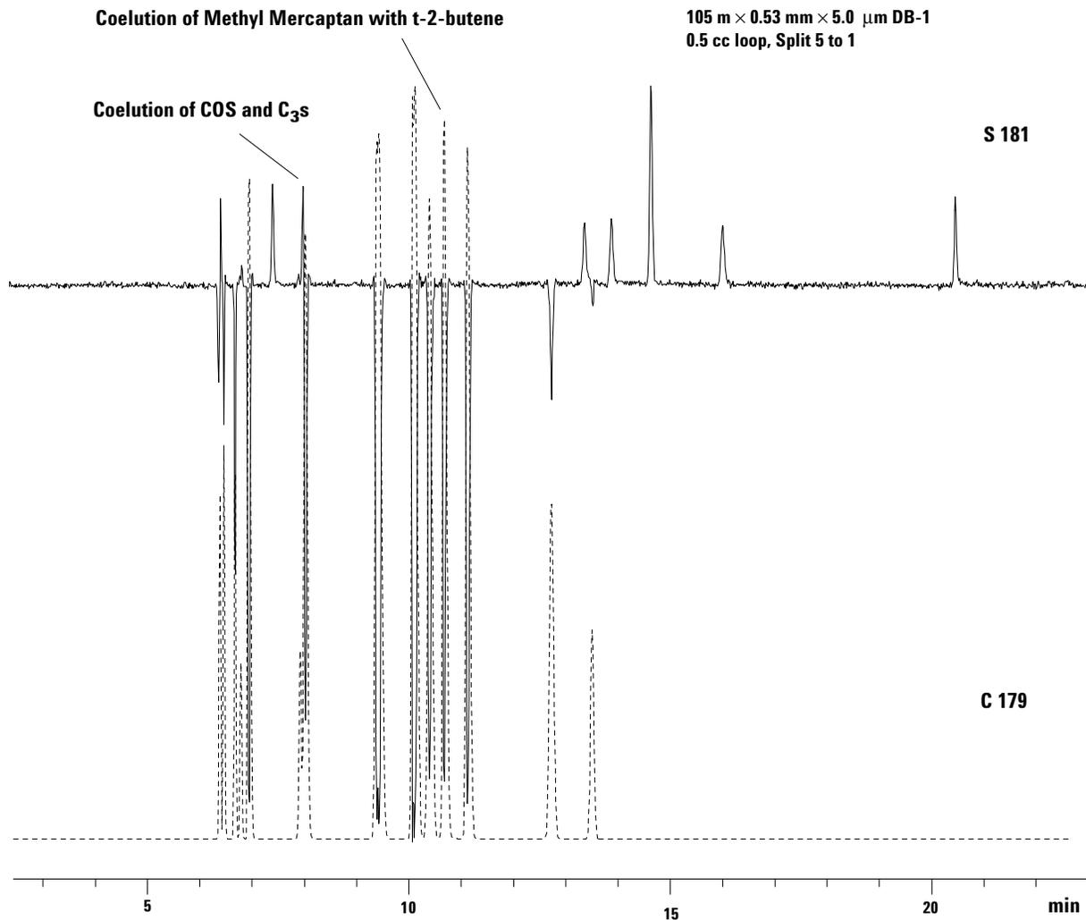
Figure 7. AED chromatograms of refinery gas blended with the sulfur calibration mix. Dashed line is carbon.
