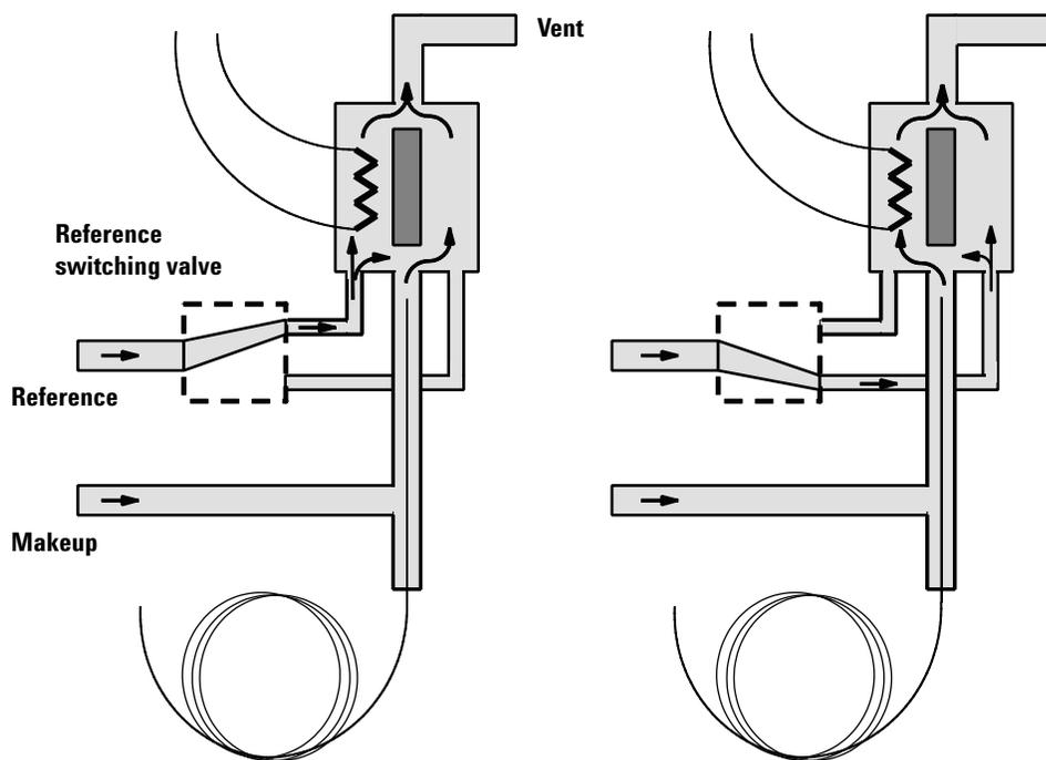
Figure 3. Pneumatic diagram of the Agilent single-filament TCD.
