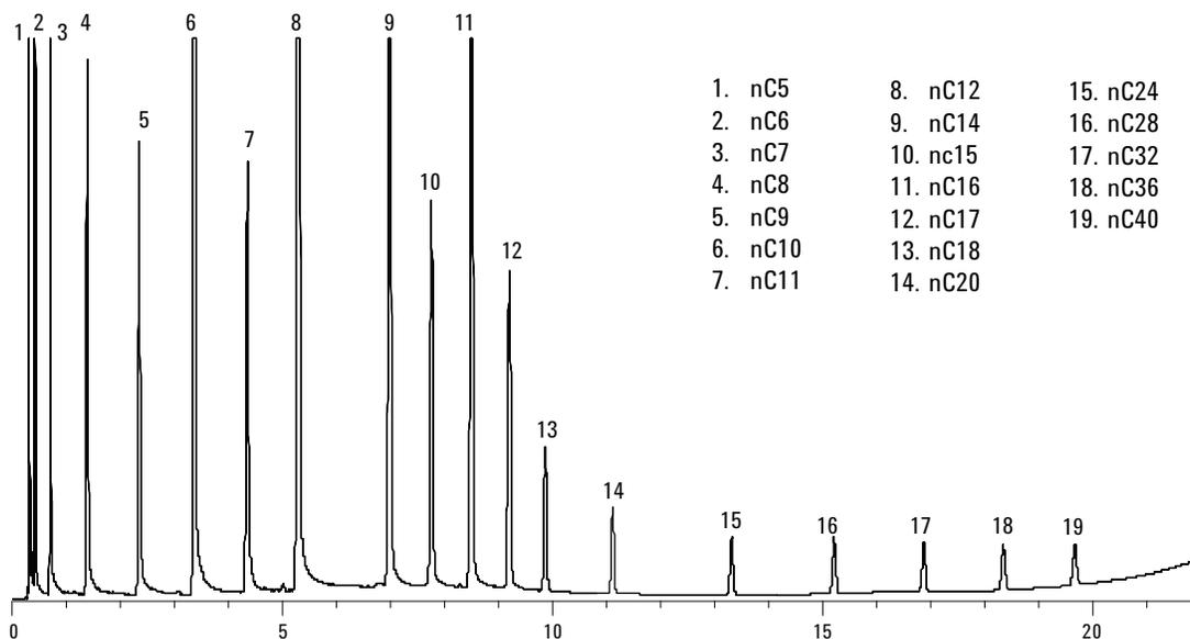
**Figure 15. Chromatogram of nC5-nC40 (D2887 BP standard diluted by CS<sub>2</sub>).**
