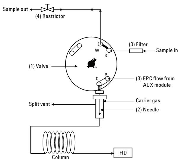
Figure 1. Flow diagram of the HPLI device.
