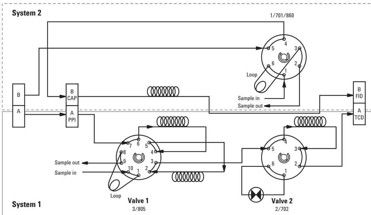
Figure 1. Valve diagram.
