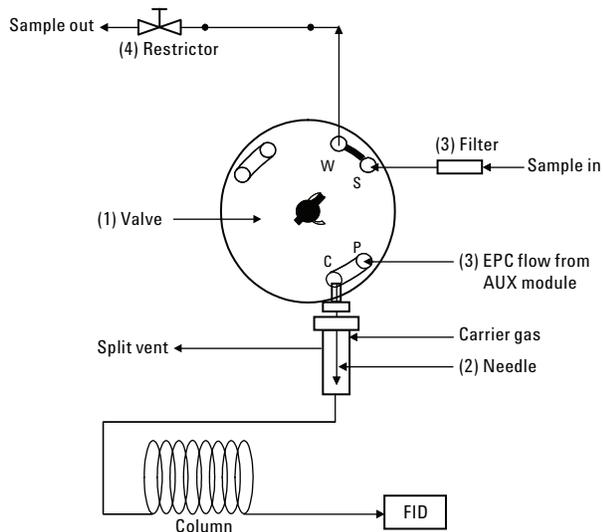
Figure 1. Flow diagram of the high-pressure injection device (HPLI).
