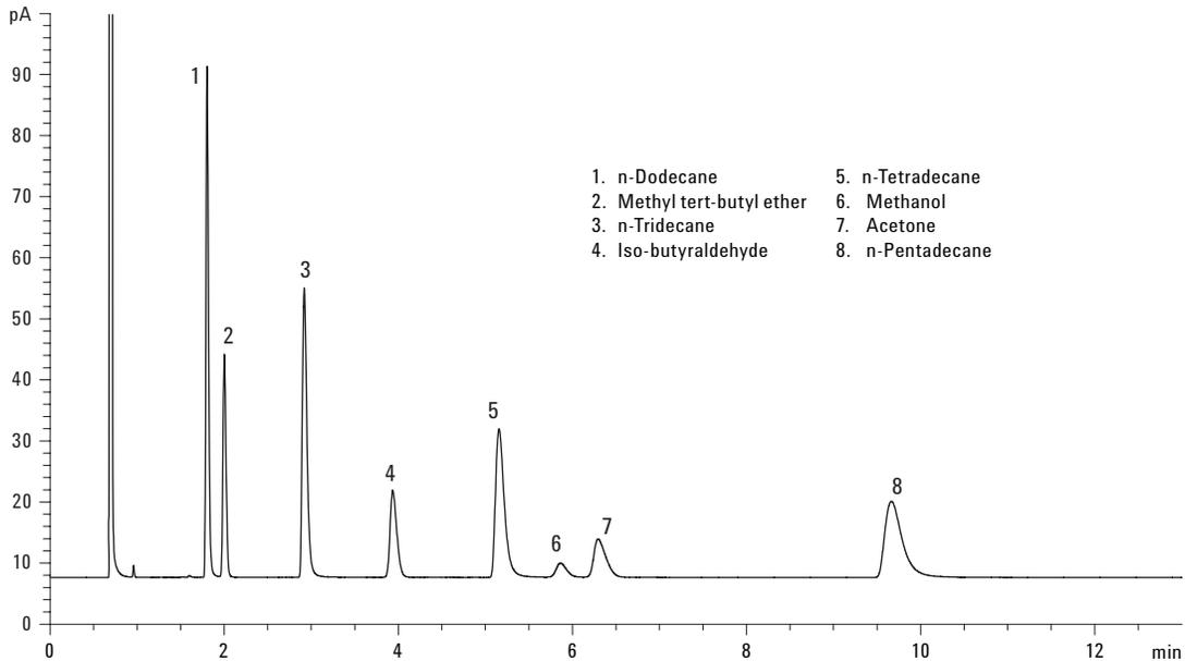
Figure 9. Chromatogram of performance mixture after 1,500 injections.
