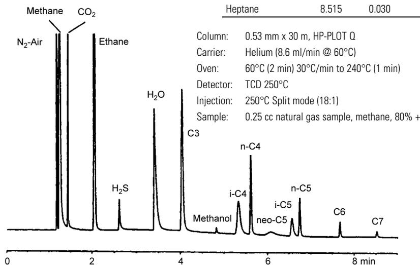
column absorbants from sample components such as water and CO<sub>2</sub> during repeated runs. Retention time shifting makes the sample timing switch more difficult and sometimes incorrect. To investigate this problem, 70 sequential runs were performed over three days. **Tables 4** and **5** list the relative standard deviations (RSDs) for the retention time averages as well as the peak ratios.
