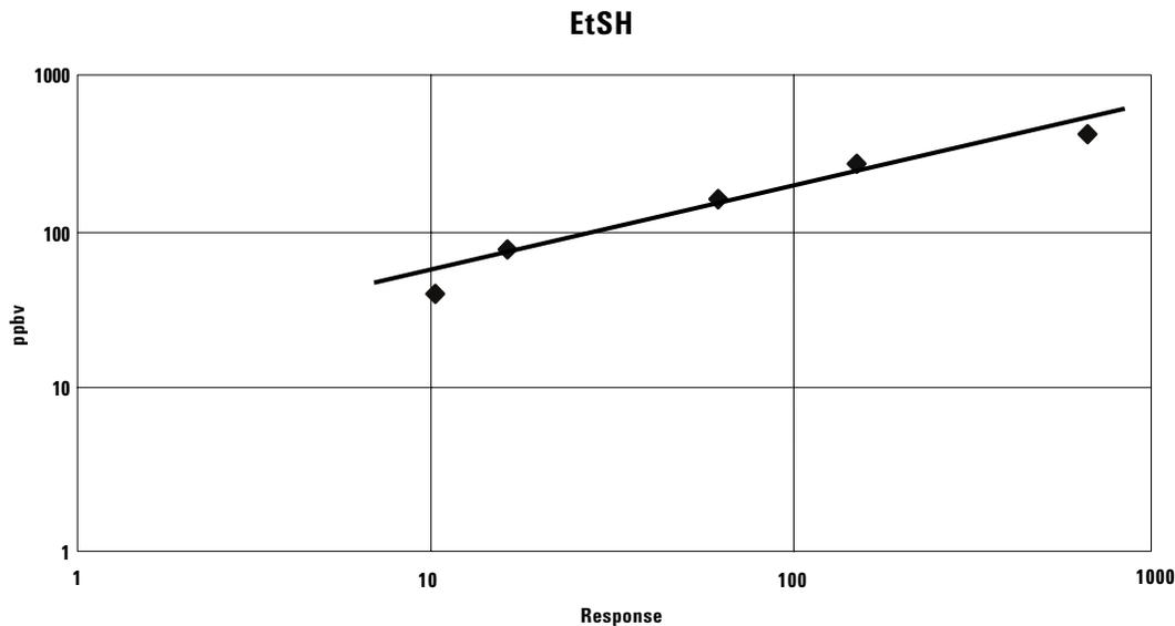
**Figure 3. Calibration of ethyl mercaptan in helium from 400 ppbv to 50 ppbv.**
