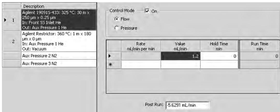
**Figure 2. Software setpoints for the analytical column.**
