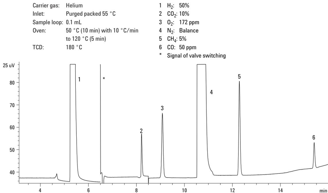
Figure 6. Chromatogram of fuel cell gas standard.
