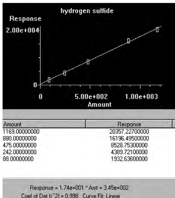
**Figure 2. Five level calibration plot of H<sub>2</sub>S using natural gas as the diluent. Calibration range is from 88 to 1170 ppb.**
