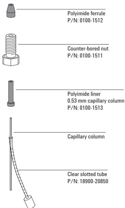
**Figure 2. Installing capillary columns using fused silica adapters.**
