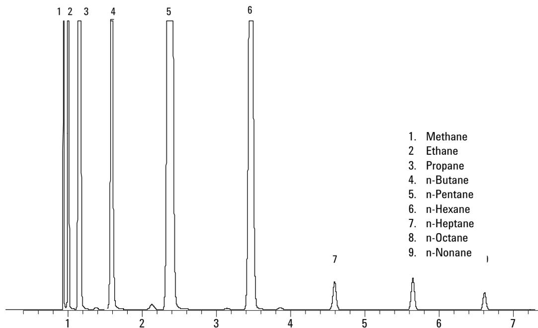
**Figure 8. Chromatogram of liquefied natural gas (calibration standard).**
