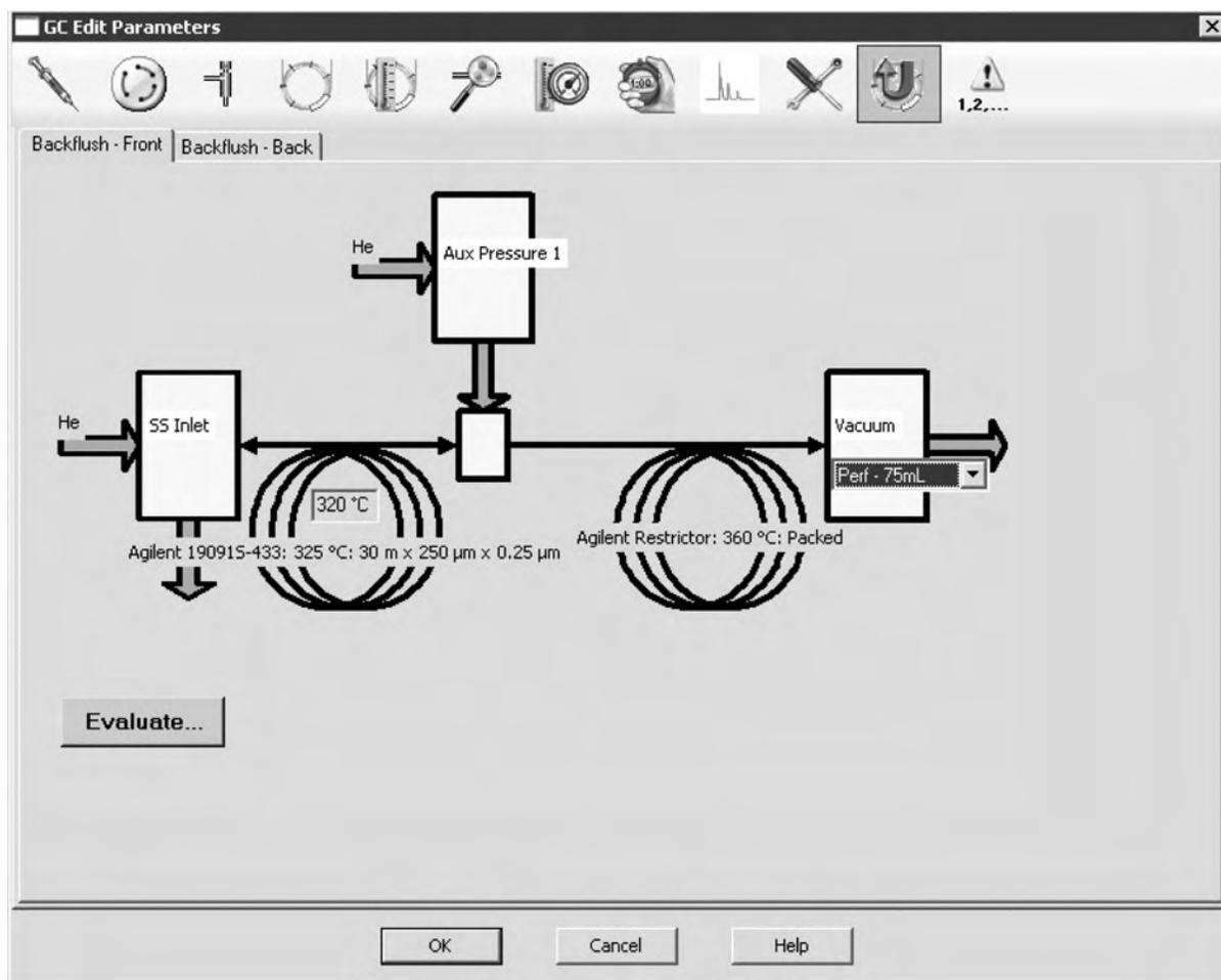
Figure 5. Interactive setup for backflush conditions in ChemStation.
