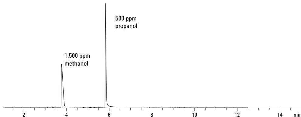
Figure 8. Test mixture of 1,500 ppm methanol in toluene.
