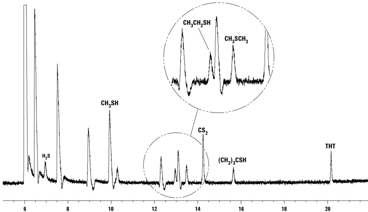
Figure 9. Sulfur mix blended with high ethane natural gas. Sulfur level: 120 ppb. Detector - Flame Photometric.
