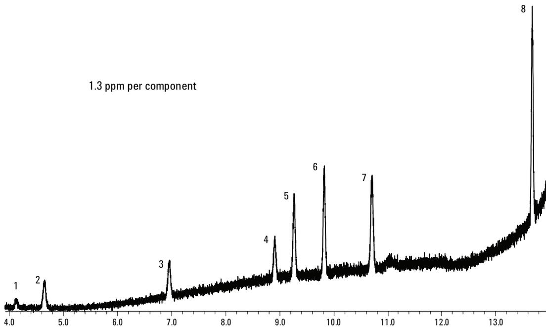
**Figure 3.** Total ion chromatogram of the eight-component sulfur mix at 1.3 ppm per component. Scan 33-100 amu. Peak labels: 1. hydrogen sulfide, 2. carbonyl sulfide, 3. methyl mercaptan, 4. ethyl mercaptan, 5. dimethyl sulfide, 6. carbon disulfide, 7. t-butyl sulfide, 8. tetrahydrothiophene.
