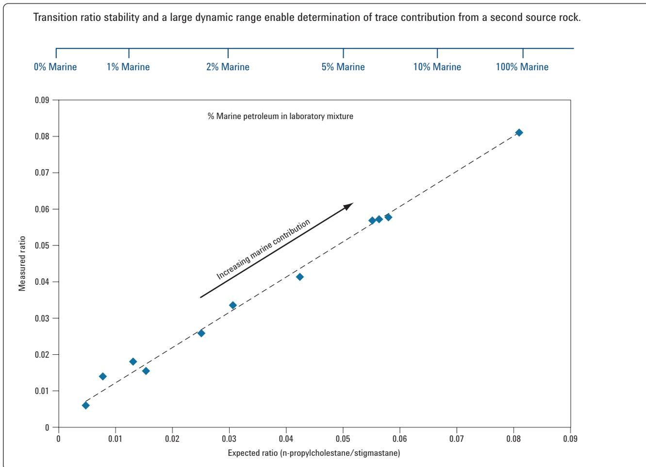
**Figure 6.** A series of laboratory mixtures consisting of various percentages of a marine petroleum sample in a lacustrine sample were analyzed for stigmastane, a ubiquitous component present in petroleum from both sources, and *n*-propylcholestane, a compound unique to oil from lacustrine source rock. The measured ratio of the two compounds was then plotted versus the expected ratio. Transitions monitored were: *n*-propylcholestane,  $m/z$  414.4→217.2; stigmastane,  $m/z$  400.4→217.2.
