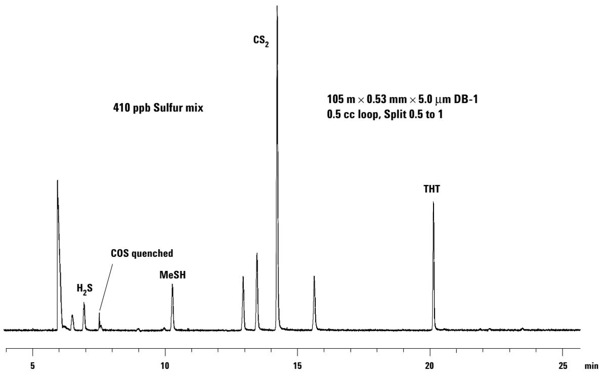
Figure 8. Sulfur mix blended with high methane natural gas at 2 ppm and 410 ppb. Detector - Flame Photometric.
