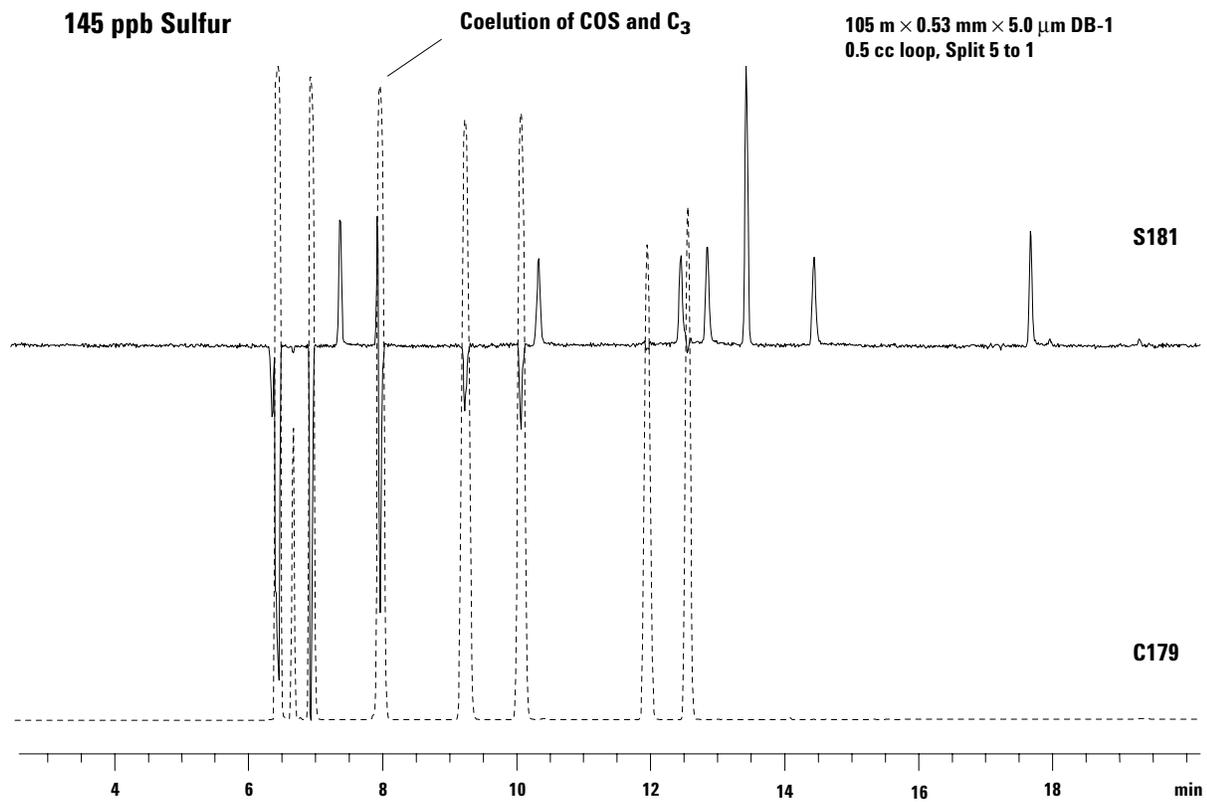
Figure 5. AED carbon and sulfur chromatograms of high ethane (9%) natural gas blended with the eight component sulfur mix. Dashed line is carbon. The carbon and sulfur chromatograms are not drawn to the same scale.
