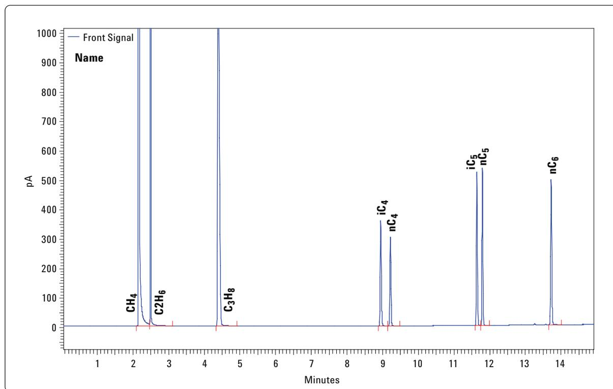
Figure 2. FID Channel chromatogram of CH<sub>4</sub>, C<sub>2</sub>H<sub>6</sub>, C<sub>3</sub>H<sub>8</sub>, iC<sub>4</sub>, nC<sub>4</sub>, iC<sub>5</sub>, nC<sub>5</sub>, and nC<sub>6</sub>.
