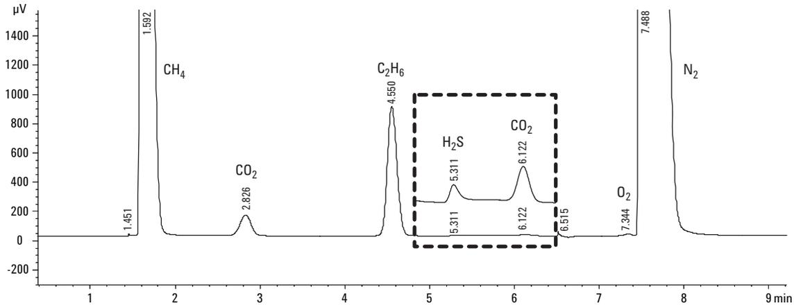
Figure 6. H<sub>2</sub>S at approximately 500 ppm and COS 300 ppm on second TCD channel.
