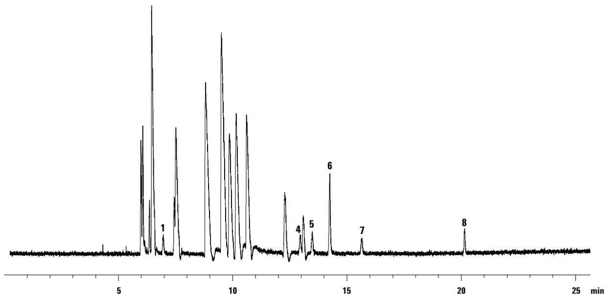
Figure 10. Sulfur mix blended with refinery gas. Sulfur level: 120 ppb. Detector - Flame Photometric. See Table 3 for peak id's.
