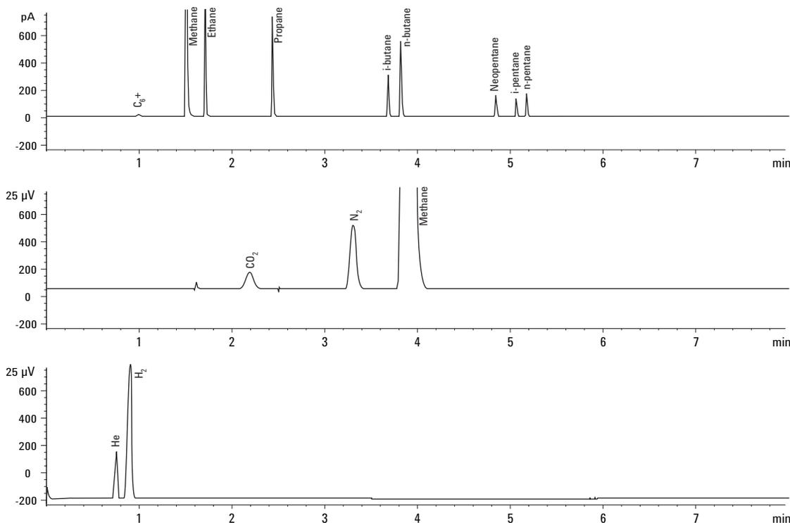
Figure 4. Natural gas analysis of a calibration gas.
