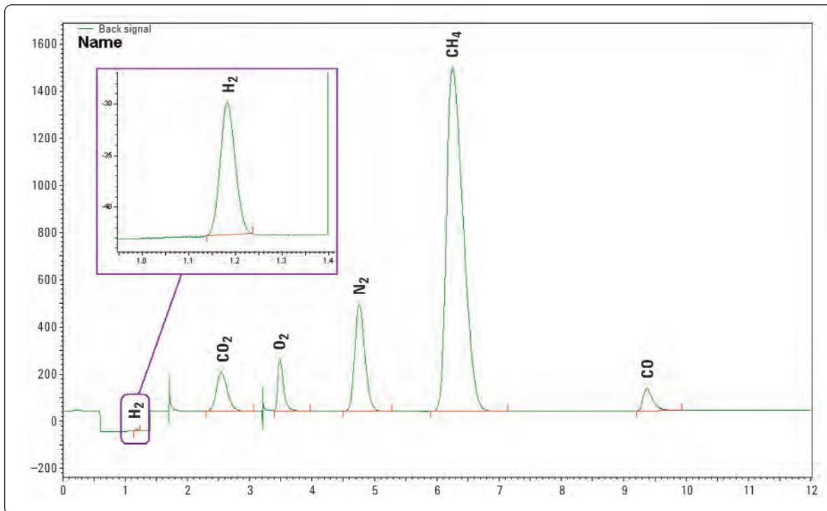
Figure 3. TCD Channel chromatogram of H<sub>2</sub>, O<sub>2</sub>, CO<sub>2</sub>, N<sub>2</sub>, CH<sub>4</sub>, CO.
