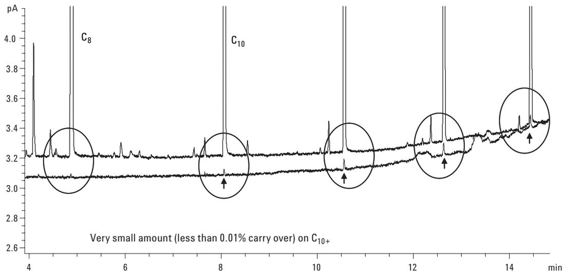
Figure 5. Carryover less than 0.01% on C<sub>10+</sub>.
