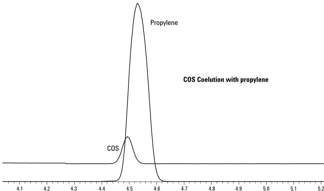
**Figure 9. Two separate chromatograms (from separate runs) superimposed showing the coelution of COS with propylene. Split ratio 50:1.**
