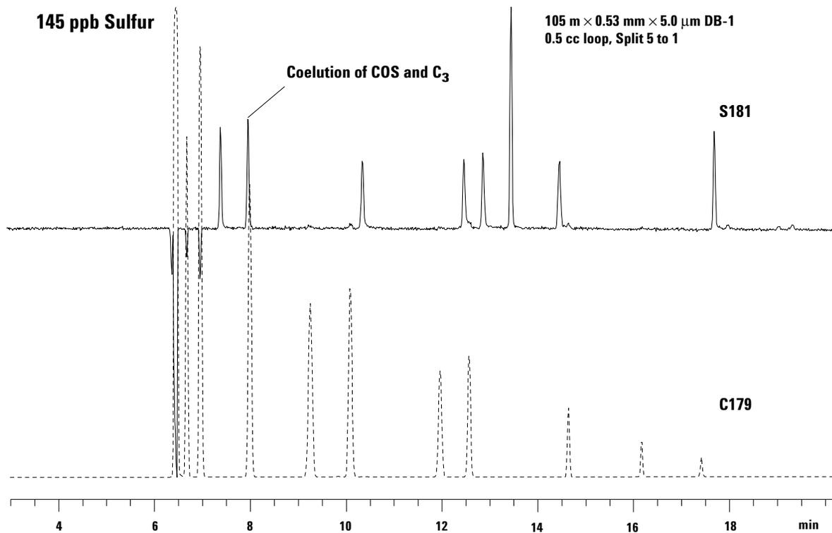
Figure 6. AED chromatograms of high methane natural gas blended with the sulfur calibration mix. Dashed line is carbon.
